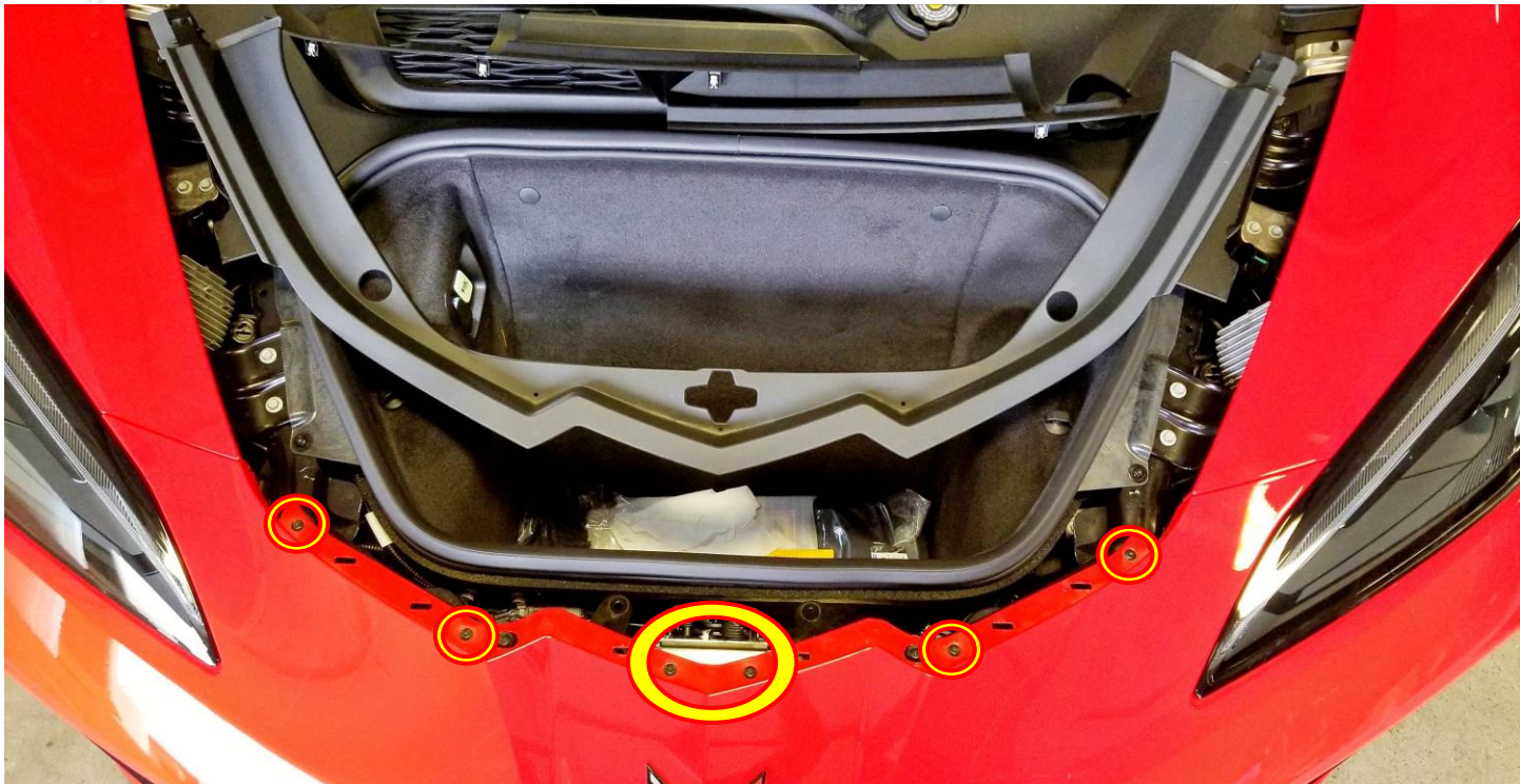
Remove all the bolts and plastic clips securing the bumper to the body and fenders. (6 on top, 1 more on each side hidden)
