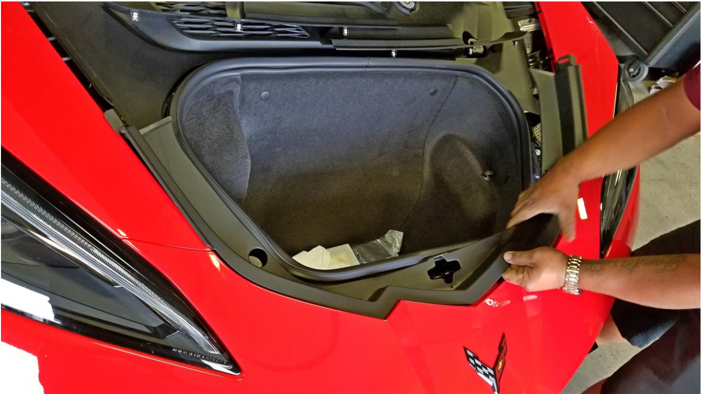
Now you can remove the panel covering the bumper bolts by pulling up on it to release clips
